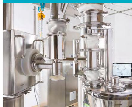
The Gericke Formulation Skid **GFS** supplies mixtures of API and up to 5 excipients within the capacity range of 1-1000 kg/h to:
